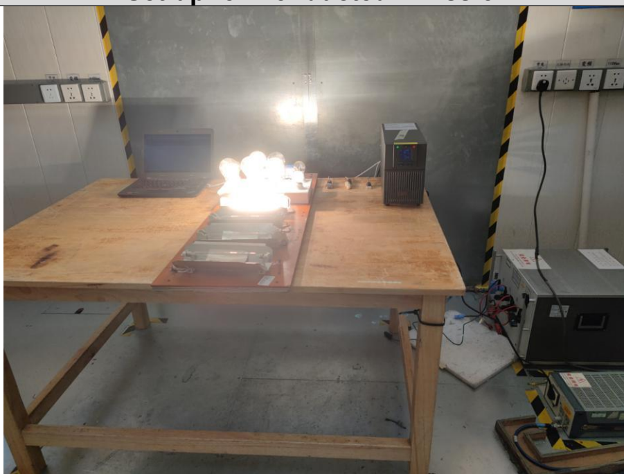
Set-up for Radiated Emission
