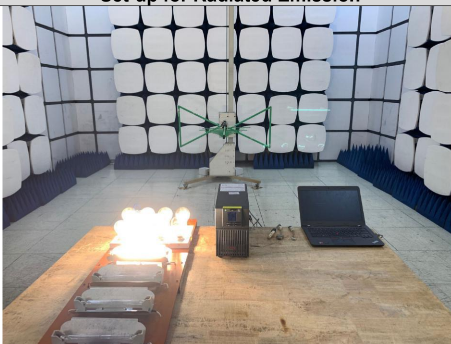
Set-up for Radiated Emission
